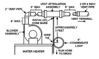
FIGURE 25: Typical Installation for Horizontal Vent with 3 or 4 inch
